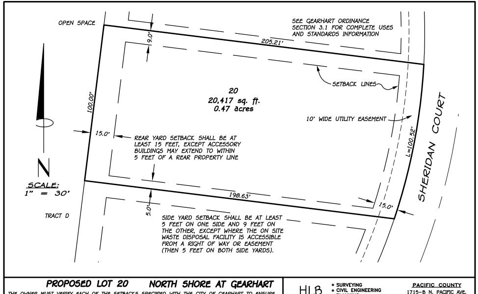
THE OWNER MUST VERIFY EACH OF THE SETBACKS SPECIFIED WITH THE CITY OF GEARHART TO ENSURE COMPLIANCE WITH ALL APPLICABLE LAND USE AND BUILDING CODES. LOT LINES, DIMENSIONS, AREA AND EASEMENTS MAY BE SUBJECT TO MINOR CHANGES AT ANY TIME PRIOR TO FINAL PLAT BEING RECORDED
